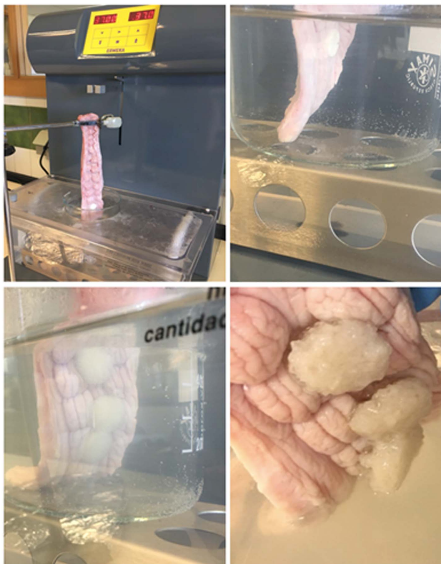
Fig. 4. Experimental device used to evaluate residence time (600 mL SVF pH 5.5 at 37 \pm 0.1 °C).
