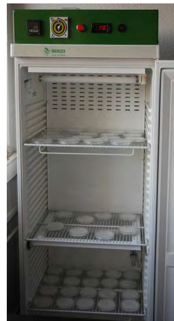
Petri dishes with seeds of various species (left) and the germination chamber used in the experiment (right).
