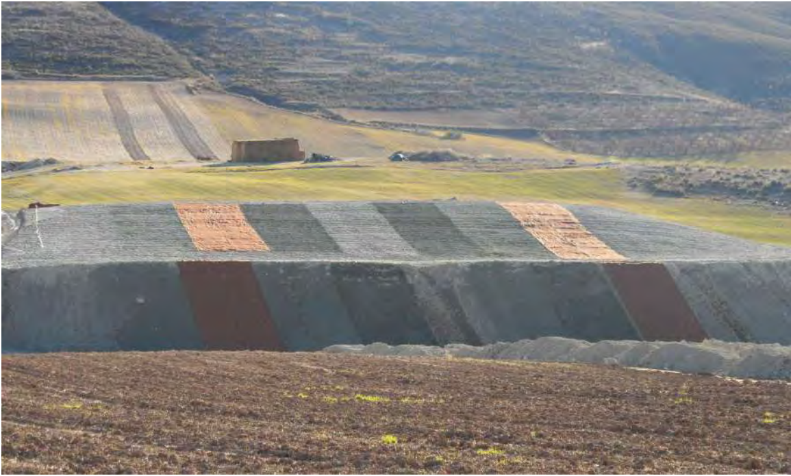
View of the experimental slopes with hydroseeding treatments distributed on two contrasting slopes: shallow (10–15%) and steep (60–65%); and two aspects: north (N) and south (S). North aspect is showed here.
