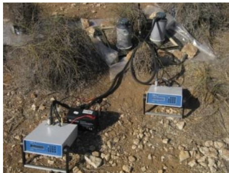
Figure 4. Soil respiration chambers in Balsa Blanca (Almería). Photograph author: Ana López Ballesteros.
