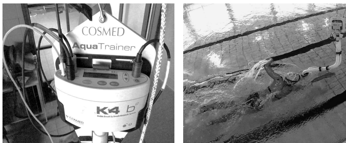
Figure 1. VO_2 assessment using the K4b 2 oximeter and the Aquatrainer respiratory snorkel and valve systems (Cosmed, Rome, Italy).
