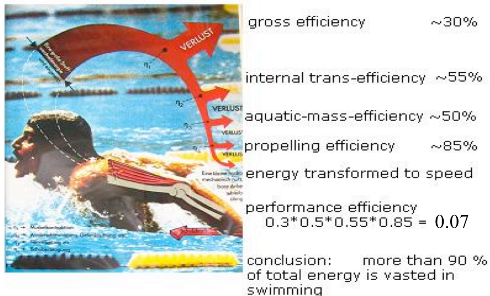
Fig.1: Efficiency-cascade of a swimmer
