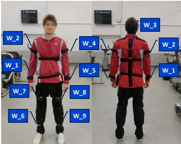
Figure 3.13: Sensor deployment for the experimental scenario. Nine MIMU-based wearable platforms ( W_1, \dots, W_9 ) are placed on different parts of the user body.
