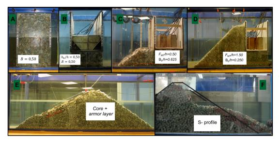
Figure 3.1.: Breakwater types tested.
