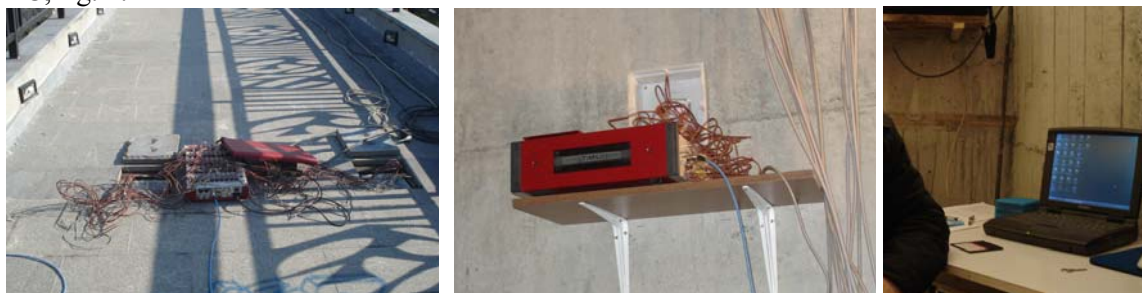
Figure 4: Switching box, data logger and saving of the date
