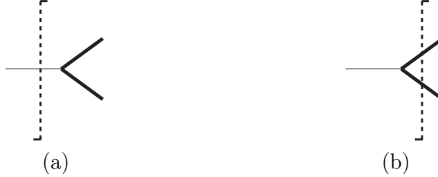
Figure 2.4: Splitting regulated by massive (thick) unobserved particles. The one-particle cut in (a) contributes to the virtual part, the two-particle cut of (b) to the real radiation.
