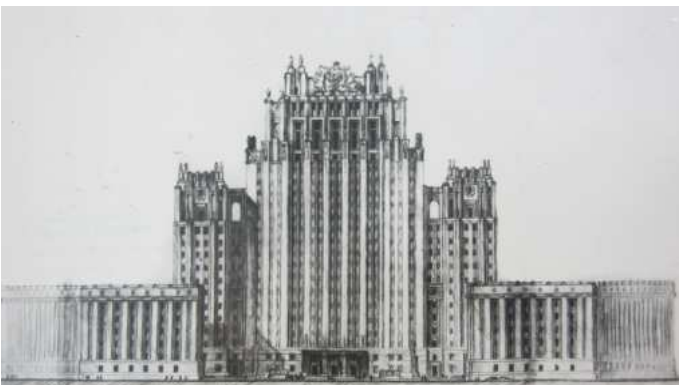
Figure 95. Moscow. Smolenskaya square. Project of high-rise administrative building. Elevation version. 1947-1948. acad. arc. V.G. Gelfreikh and arc. Minkus M.A. 20 floors. Metal framework.
