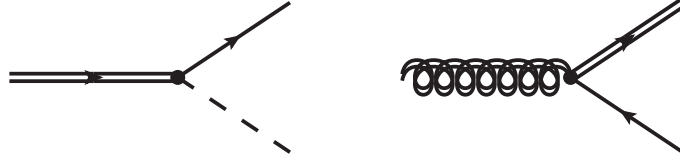
Figure 4.3: Left: Decay of a heavy quark into a SM quark and the Higgs boson. Right: Decay of a heavy gluon into a SM quark and its heavy partner.
