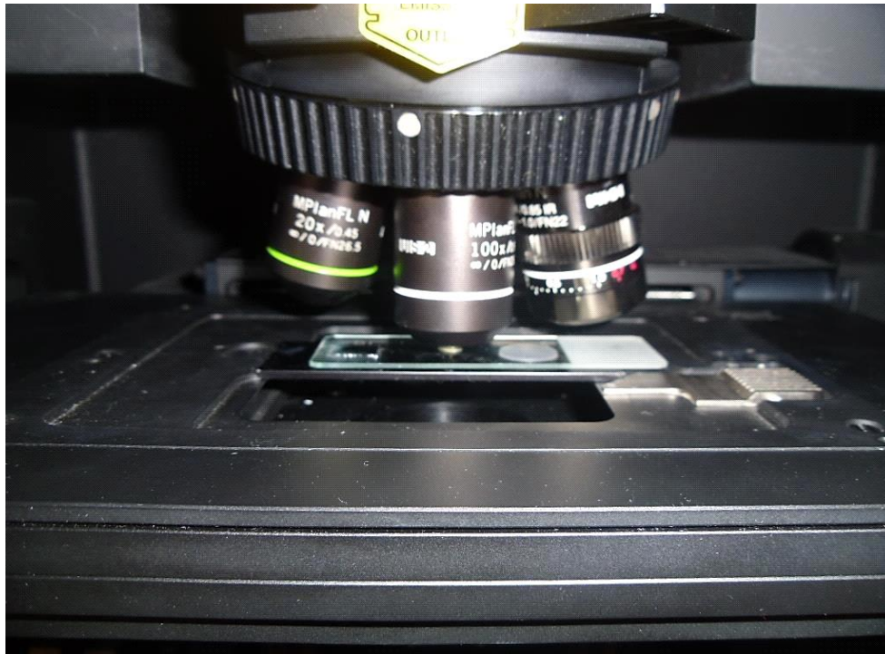
Figure 29: The sample was placed on a glass slide and focused under an X100 microscopic objective lens
