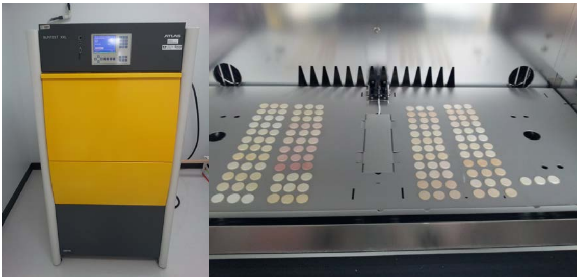
Figure 6.5: ATLAS Suntest XXL artificial aging device at HCBB (left) and placement of the sample inside the artificial aging chamber (right).
