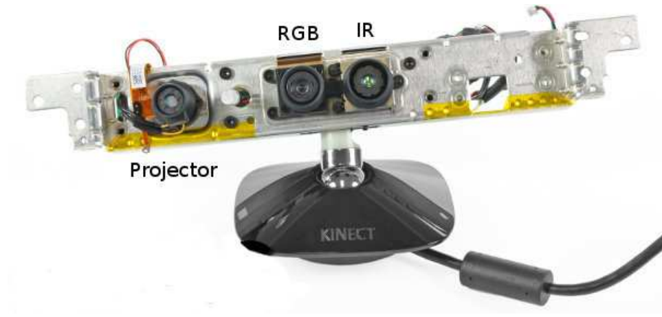
Figure 5.2: Kinect consists of infrared emitter, infrared sensor and RGB camera, as well as microphones and tilt motor. (Illustration from [129]).
