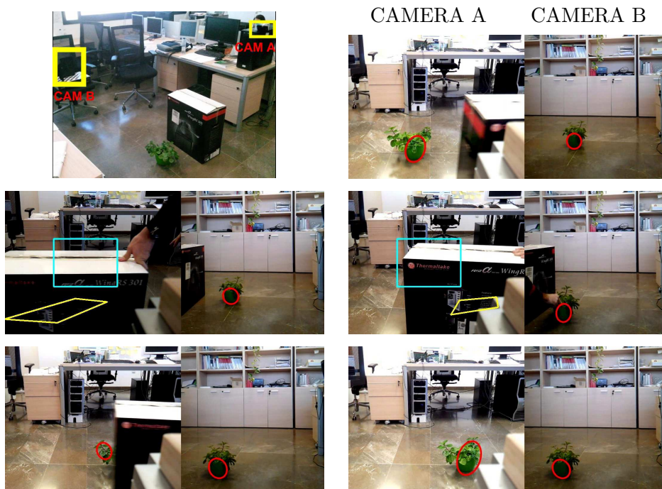
Figure 6.14: Behavior of the tracking in the presence of occlusions. The object is completely occluded in camera A , depending the tracker on remote information provided by camera B . Movements of the object are tracked by camera B and forwarded to camera A , allowing it to update the object's location and the search window of the CAMSHIFT tracker. Thus, the object is located and tracked in the first moment that it becomes visible again.
