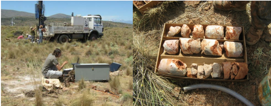
Figure 5. Left, doing the borehole in Llano de los Juanes. Right, rock cores.
