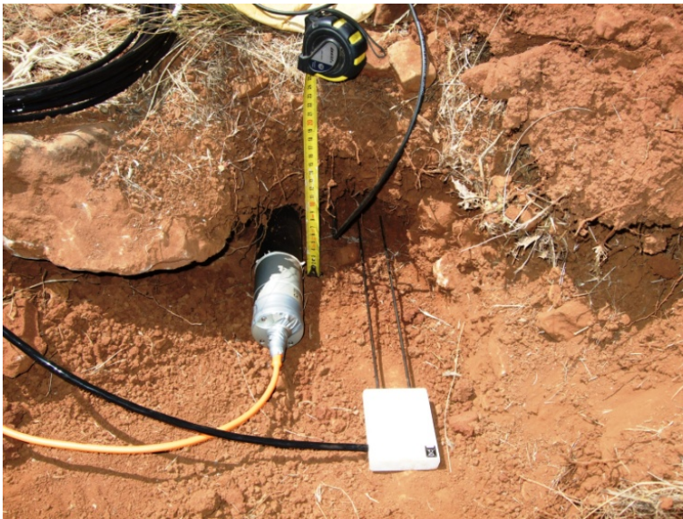
Figure 4. Installing CO 2 sensor, soil water content and temperature probe.
