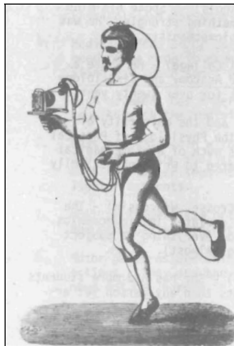
Figure 2.1.4. Man in action carrying a device to record pressure vs. ground and vertical movement of the head. (Marey, E.J., La Machine Animal , Felix Alcan, Paris, 1886)
