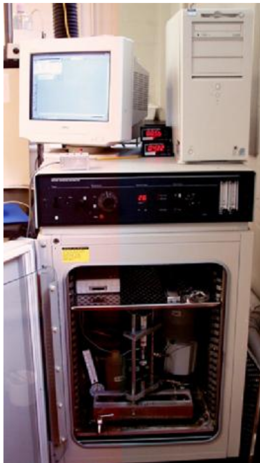
Figure A1- 12. Home made beam bender apparatus and equipment in the incubator.
