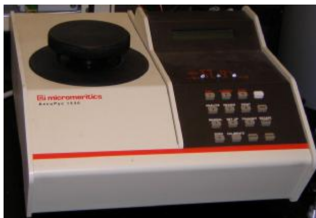
Figure A1- 19. Picture of the Helium Pycnometer.
