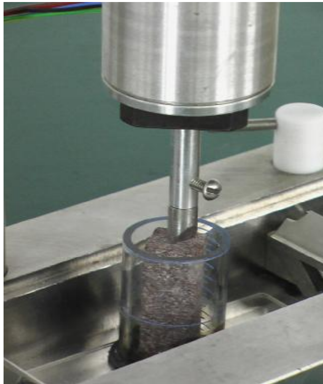
Figure A1- 9. Detail of the pushrod tip and LVDT used for measuring the free swelling of stone sample, which was placed in a glass container.
