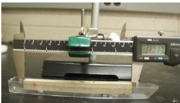
Figure A1- 10. Caliper set-up for quick measurements of swelling.
