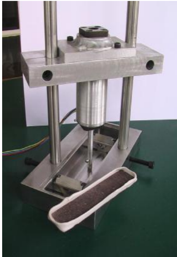
Figure A1- 24. Warping device set up. Detail of the sample preparation before pouring the water. The perimeter of the sample is surrounded with a sealant material in order to keep the water on the top surface during the whole test.
