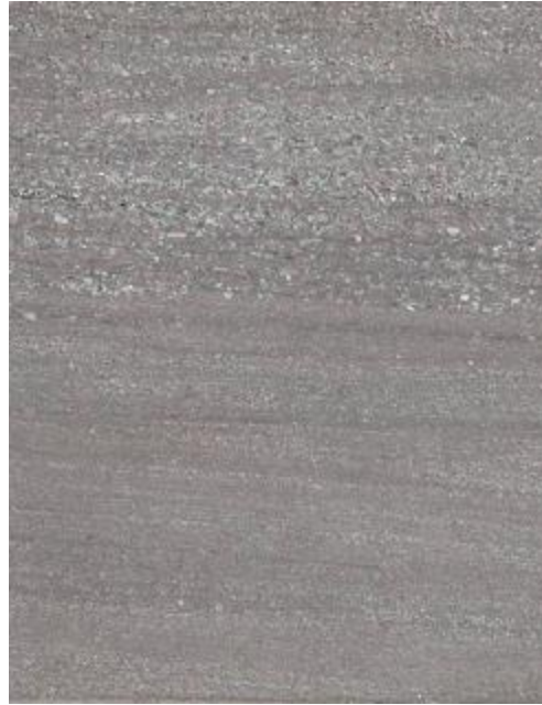
Figure 4-5. Illustration of Portland Brownstone heterogeneity and anisotropy
