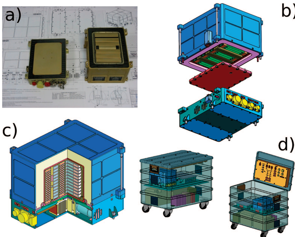
Figure 1. The GCF-2. (a) Photograph of the GCF-2 filled with modules and of the EU. (b) Schematics of the mounting of the GCF-2. (c) Schematics of the layout of the crystallization reactors inside the GCF-2. (d) Schematics of the GSE.
