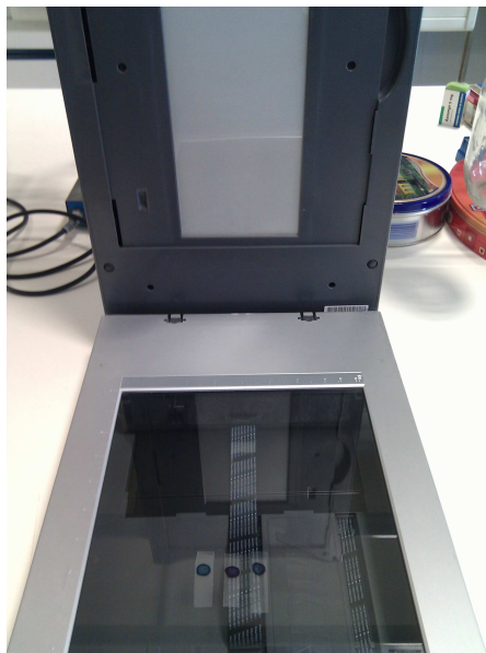
Figure 2. Scanner used to imaging the sensing membranes in transmission mode
