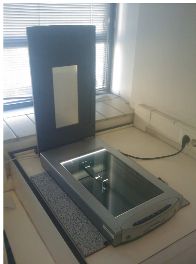
Figure 2. Acquisition of analytical signals from optical tongue by scanner working in transmission mode.
