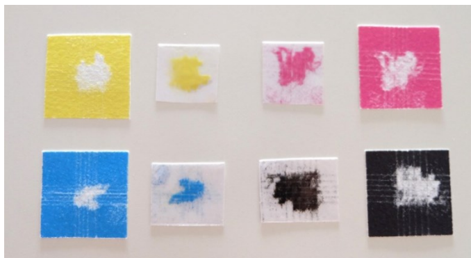
Fig. 2. View of the samples serving to determine the degree of ink adhesion
