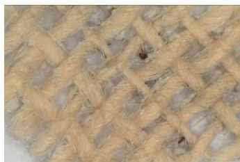
Fig. 21. Textile sample (cotton) of T-MAP1. Olympus SZH10 (3x)
