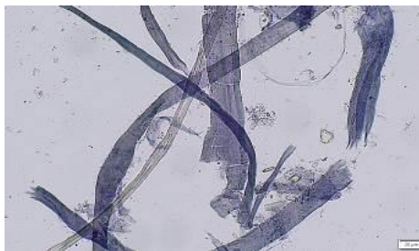
Fig. 4. Mixture of herbaceous flax and hemp fibres of P-MAP8. Olympus Vanox AHMTX (10x).
