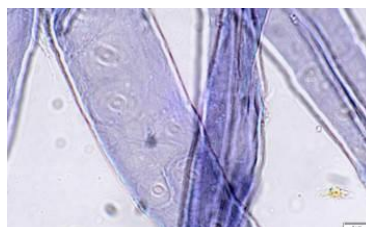
Fig. 18. Typical areolated pit of conifers of P-MAP13. Olympus Vanox AHMT3 (50x)
