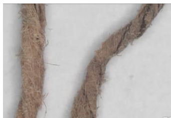
Fig. 23. Wood fibres compressed into the textile of T-MAP14. Olympus SZH10 (3x)
