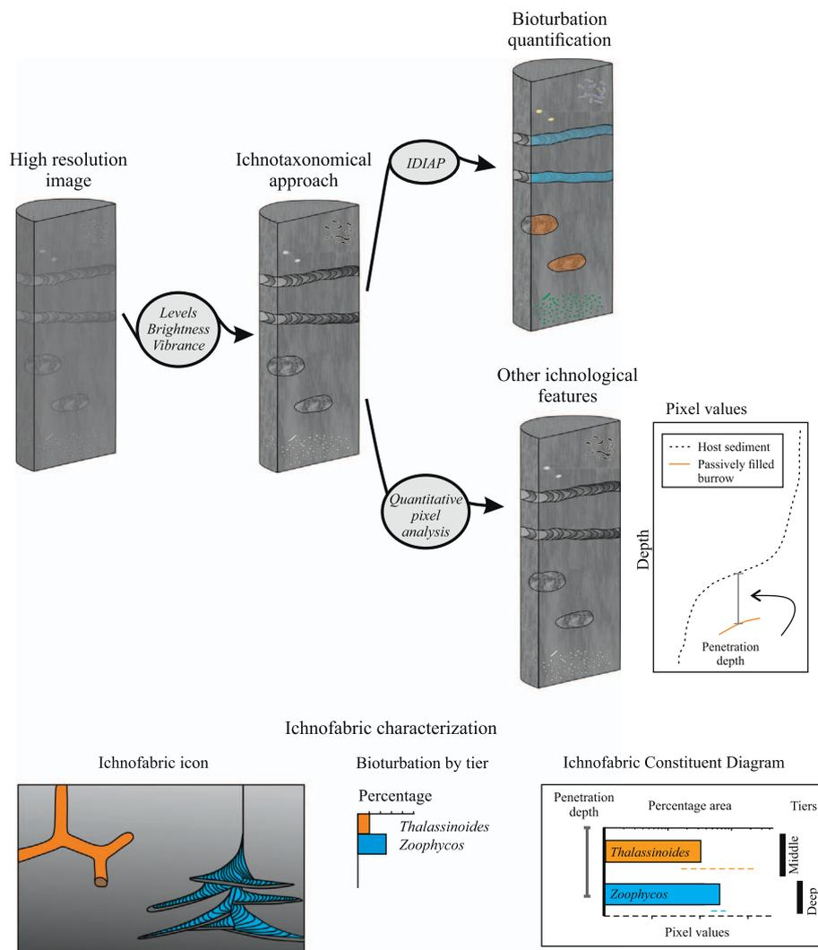
Fig. 1. Schematic diagram of the developed high resolution image treatment.
