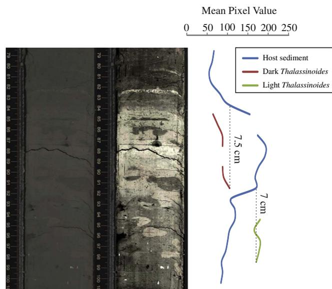
Fig. 4. Penetration depth of dark (red) and light (green) *Thalassinoides* in the U1385E-17H-3-A core. To the left, original and treated images. (For interpretation of the references to color in this figure legend, the reader is referred to the web version of this article.)
