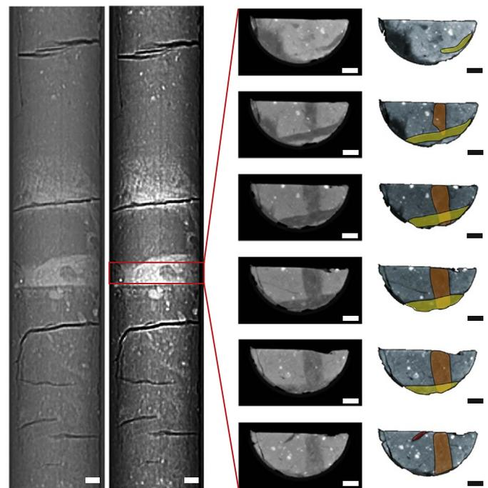
Fig. 8. Original and treated image from an interval of Site U1308 core (drilled in Hudson Strait), where Heinrich Stadial 1 can be detailed analyzed, and treated sections where overlapping situation can be clearly identified with the study of CT transversal sections. Scale bars 1 cm.
