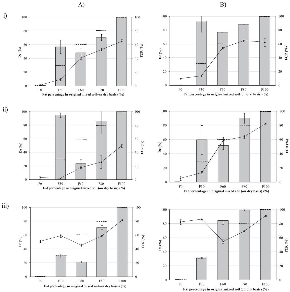
**Fig. 4.** In Figures 4, "a)", "b)" and "c)" should be removed from the bottom of the figures. Thank you Influence of pH on the cleaning of fat/starch mixtures. Cleaning maps of De and FCR at 40 °C (column A) and 50 °C (column B) pH: 3.0 (i), 7.0 (ii) and 13.2 (iii). Solid line = De values, dashed segments = fat rate in the original mixed deposit; bars = FCR values. Cleaning time 10 min, flow rate 120 L/h (error bars represent  $\pm$ SD of at least 3 measurements).
