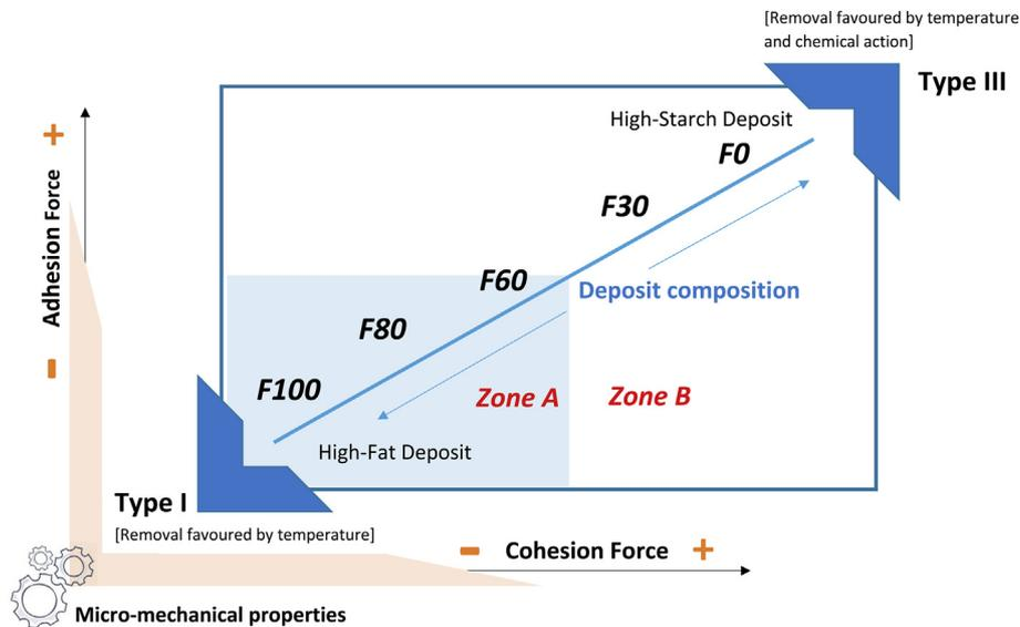
**Fig. 7.** Cleaning map. Micro-mechanical approach for the deposits removal as a function of their fat fraction (%) and the recommended cleaning conditions. In the graph are defined deposit type 1 and 3 as zones of specific adhesive/cohesive interactions.
