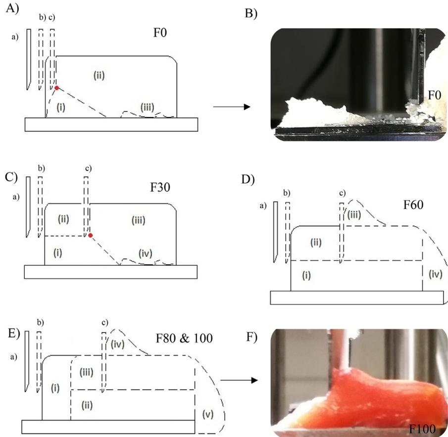
**Fig. 2.** Schematic mechanical behavior for each type of deposit depending on its base composition. Blade position during the mechanical removal: points of interest represented by a) b) and c).
