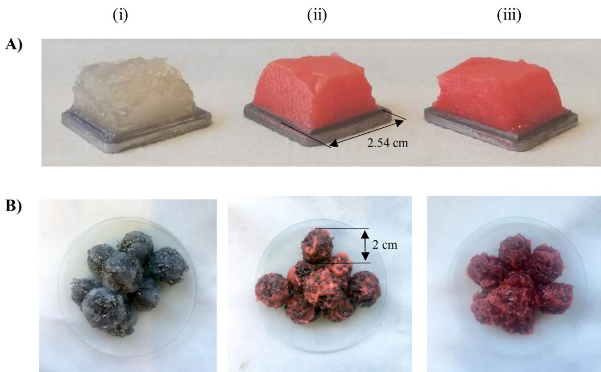
**Fig. 1.** Stainless steel flat (A) and spherical coupons (B) soiled with (i) gelatinised starch (F0), (ii) mixed deposit with 60% (w/w) fat on dry basis (F60) and (iii) colored pork lard (F100).
