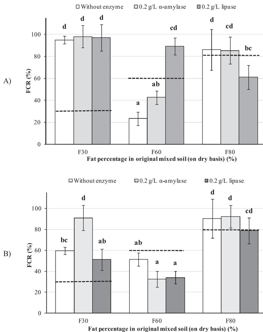
**Fig. 6.** Influence of enzyme addition on the FCR of fat/starch mixtures. Cleaning maps at 40 °C (A) and 50 °C (B). Dashed segments = fat rate in the original mixed deposit; bars = FCR values. pH = 7, cleaning time 10 min, flow rate 120 L/h (error bars represent  $\pm$ SD of at least 3 measurements). Different letters denote statistical differences between the experimental conditions using the Fisher's Least Significant Difference test with a 95.0% confidence level.
