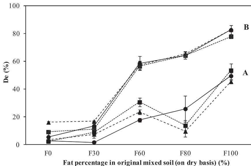
**Fig. 5.** Influence of enzyme addition on the detergency of fat/starch mixtures. Cleaning maps at 40 °C (A) and 50 °C (B). ● without enzyme, ▲ 0.2 g/L  $\alpha$ -amylase, ■ 0.2 g/L lipase. pH 7.0, cleaning time 10 min, flow rate 120 L/h (error bars represent  $\pm$ SD of at least 3 measurements).
