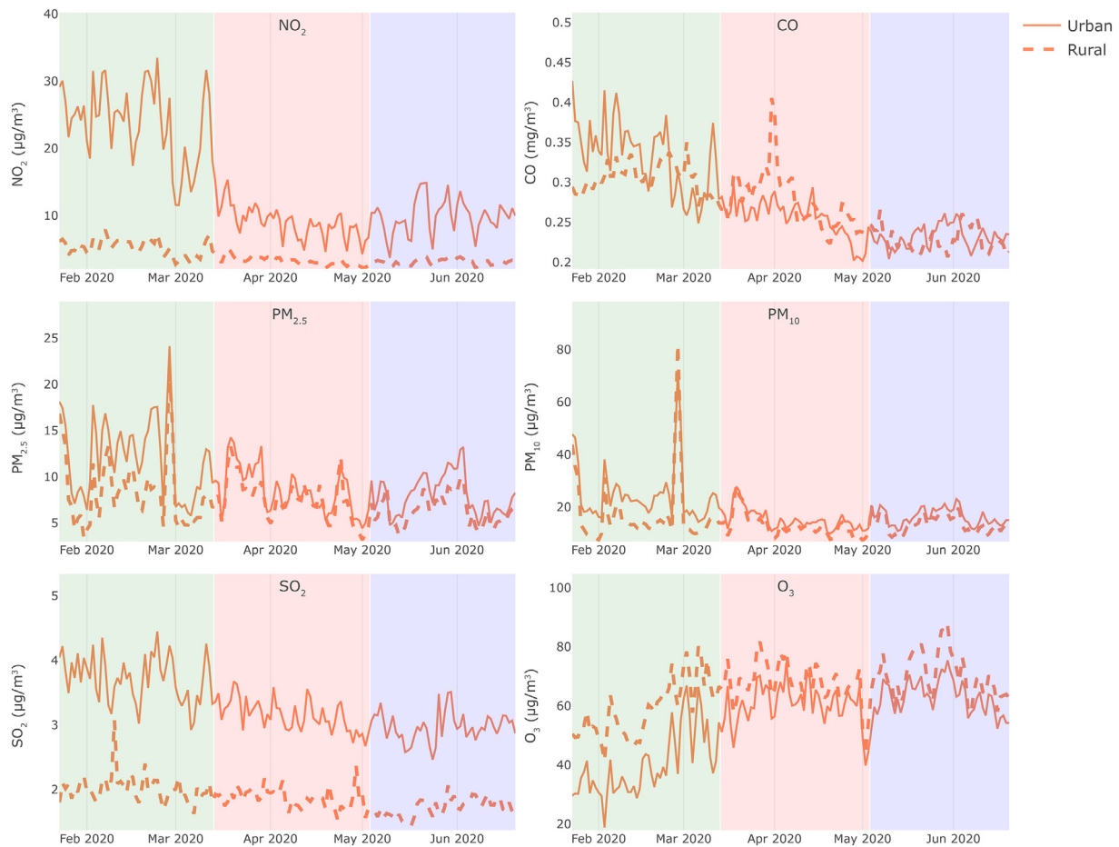
Fig. 2. Average pollutants levels in Spain across time during the three periods of the COVID-19 pandemic. Green, red and blue backgrounds represent prior to lockdown, strict lockdown and relaxed lockdown periods respectively.
