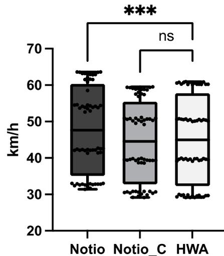
**Figure 4.** Comparative boxplot between Notio, Notio\_C, and HWA wind speed (WS), including medians, interquartile ranges, and outliers, with statistical significance analysis: ns, non-significant; \*\*\*  $p < 0.001$ . Created with GraphPad Prism 10.
