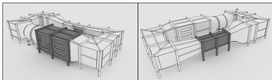
**Figure 1.** Three-dimensional representation of the wind tunnel, with the two test sections shaded, the low-speed test section on the left and the high-speed test section on the right. Original image of the wind tunnel manual with permission (Oritia & Boreas).
