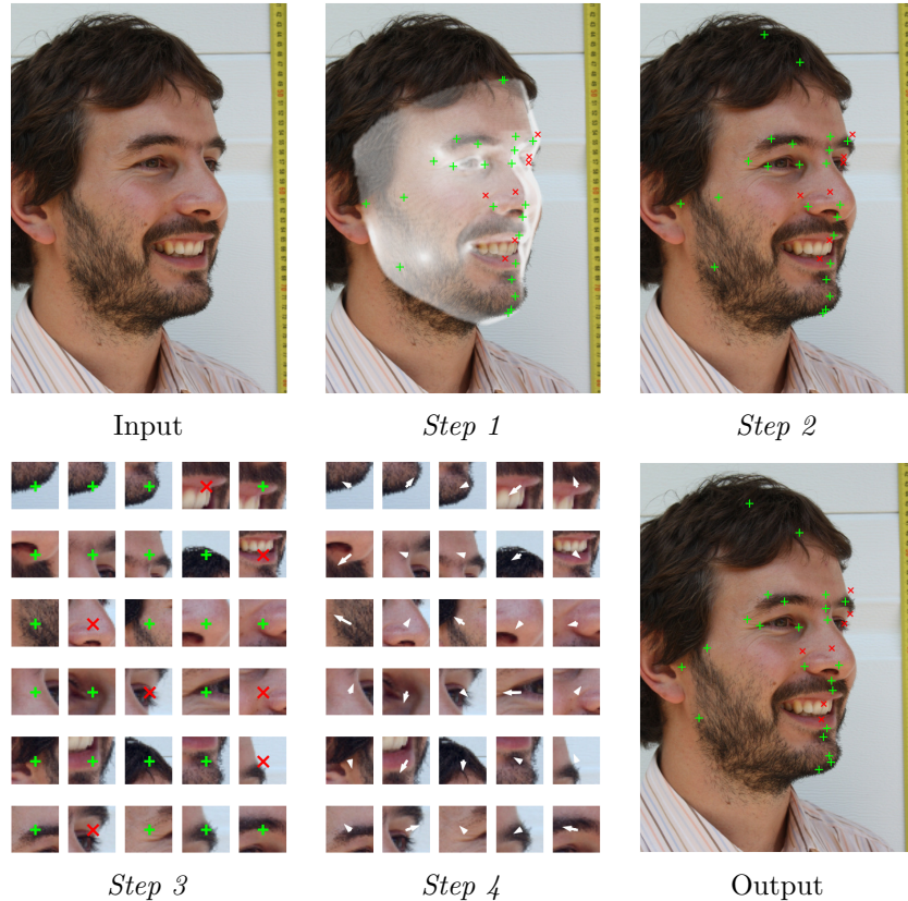
Figure 17: Full process step by step as described in Section III.3.2 (zoom in for details). Notice the different crop sizes depending on the landmark as well as the significant improvement in accuracy.
