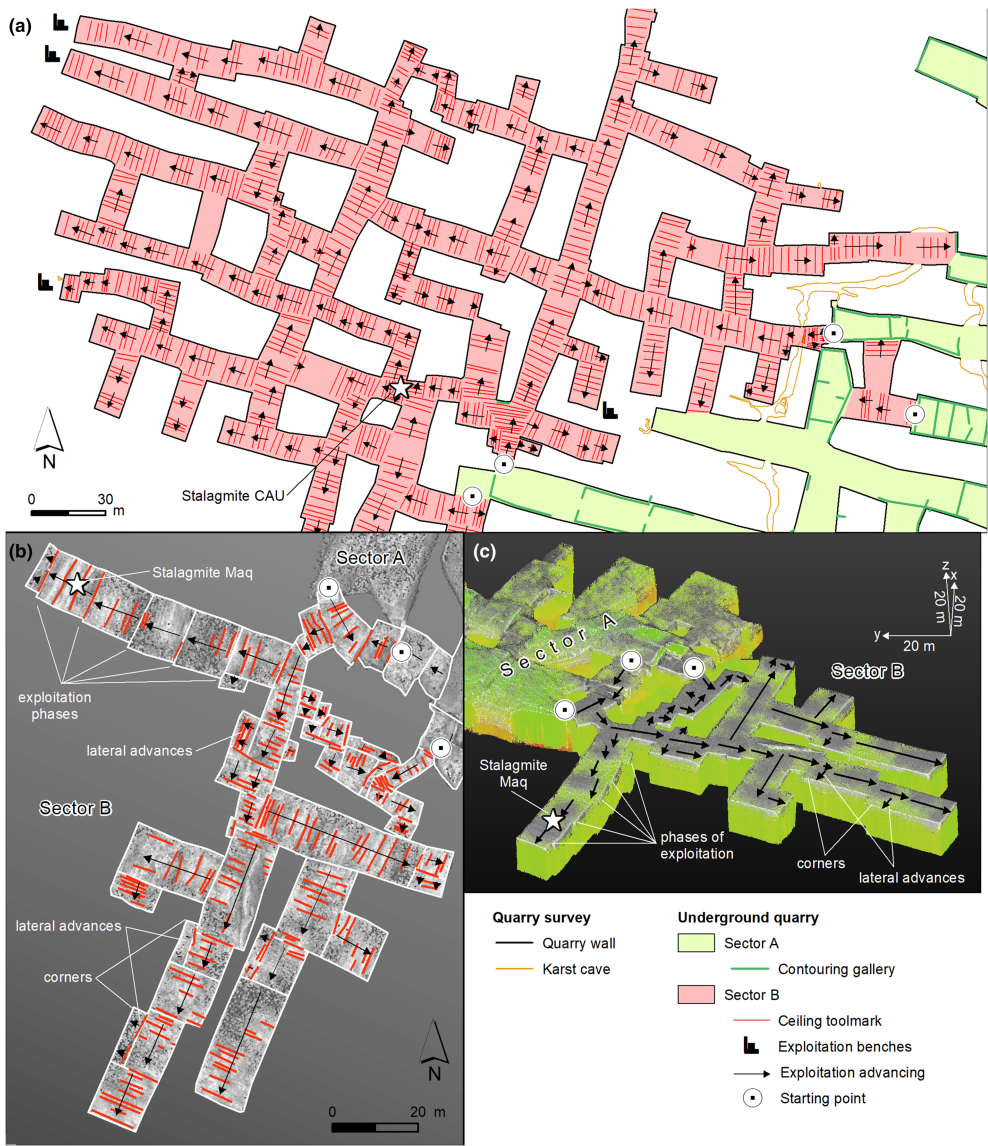
FIGURE 3 (a) West part of the quarry map showing ceiling toolmarks, excavation progress and examples of exploitation phases and corners. (b) Ceiling toolmarks shown by the high-resolution 3D model, indicating the direction of the exploitation in Les Maquisards part. (c) 3D geometry of the galleries. The starting points of sector B are indicated (white dots) in the three sections, the positions of which are shown in Figure 2A [Color figure can be viewed at wileyonlinelibrary.com ]
