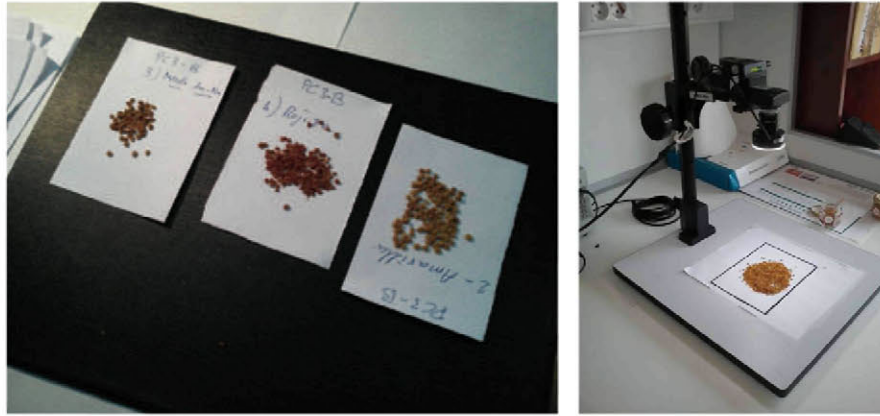
Fig. 2. On the left, some separated pollen load samples are shown. On the right, the computer vision system used to get images is presented.
