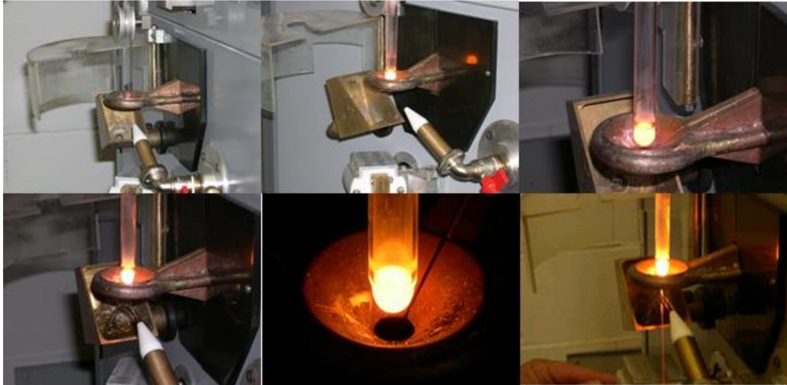
**Amorphous microwire fabrication process**
