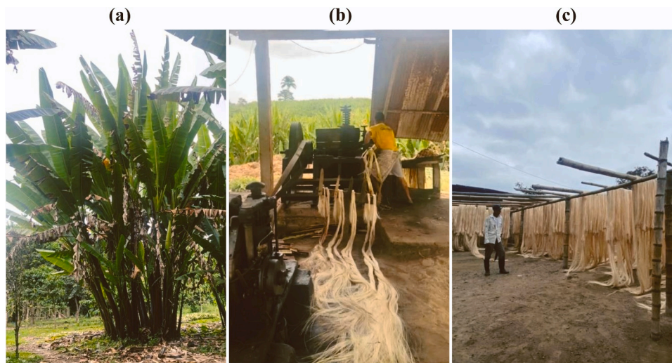
Fig. 3. Abaca fiber production stages in Santo Domingo-Ecuador: (a) group of abaca trees, (b) stripping process, and (c) drying process.
