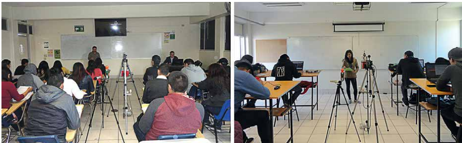
Figure 4. Application of surveys in the evaluation indoor spaces. Left. Classroom with people sitting (heights: 0.1, 0.6, and 1.1 m). Right. Drawing workshop with people semi-sitting (heights: 0.1, 0.85, and 1.4 m).
