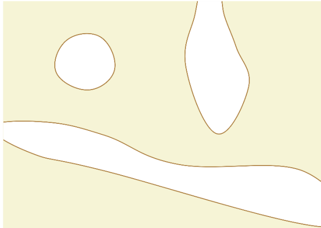
Figure 20. Scheme of different pore shapes. Porous materials present different kind of behaviour for fluid mechanics depending if they are: closed, dead-ended or opened at both sides. This effect cannot be measured by porosity ratio.
