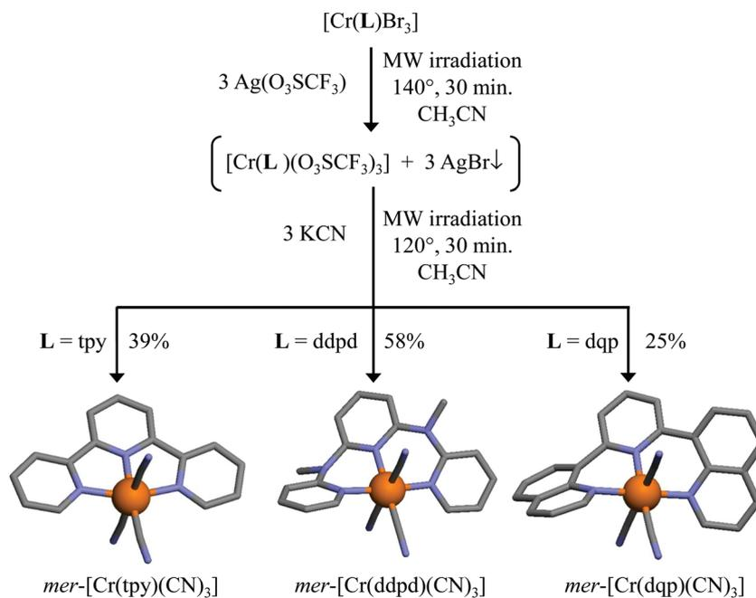
Fig. 3 Syntheses and structures of  $\text{mer-[Cr(L)(CN)}_3]$  (L = tpy, ddpd, dqd). Color code: C = grey, N = blue, Cr = orange. H atoms have been omitted for clarity.
