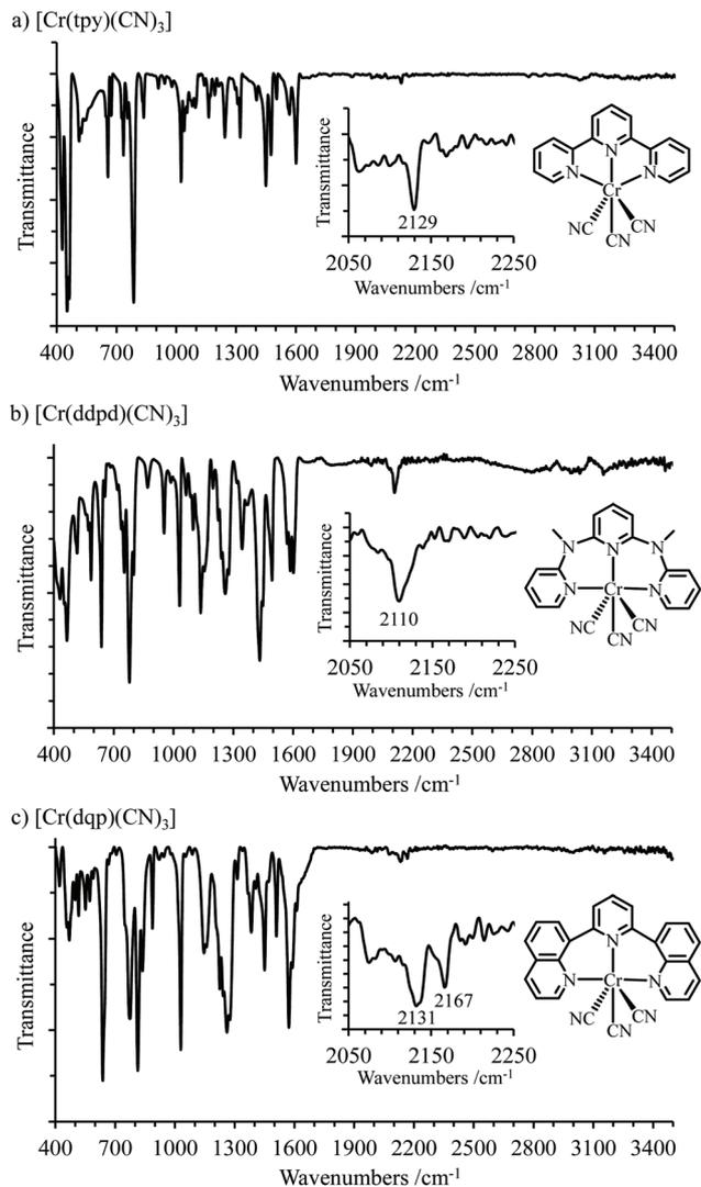
Fig. 4 IR spectra of *mer*-[Cr(L)(CN)<sub>3</sub>] (L = tpy, ddpd, dqp) recorded in the solid state at 293 K.
