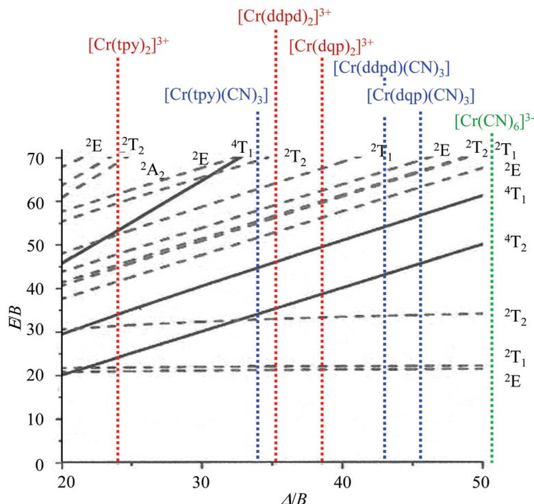
**Scheme 2** Tanabe–Sugano diagram for the  $d^3$  configuration in an octahedral ligand field (computed for  $C/B = 4.5$ ) highlighting the pseudo-octahedral  $[\text{CrN}_6]$  (red),  $[\text{CrC}_3\text{N}_3]$  (blue) and  $[\text{CrC}_6]$  (green) chromophores.  $\Delta/B$  taken from Table 2.
