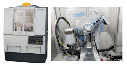
**Figure 36.** X'pert Pro θ-θ system in reflection Bragg-Brentano geometry for powder measurements. Petrology and Mineralogy Department, Facultad de Ciencias, UGR.
