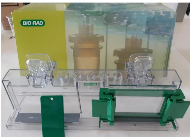
**Figure 5.1** BIO-RAD casting cells and glass and short plates for shaping hydrogel into sheets.
