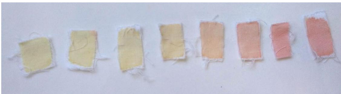
**Figure 3.13** Color change of the AD-VS indicator immobilized on cloth depending on the pH.
