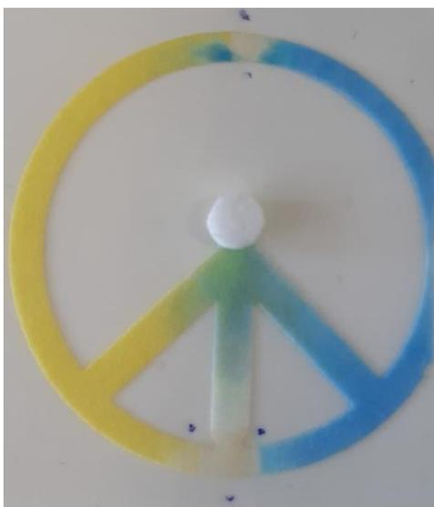
**Figure 5.16** *Second example the use of NIPAM ionogel barriers within a  $\mu$ PAD.*
