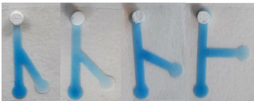
**Figure 5.18.** Different angles tried for the second channel in the  $\mu$ PAD.
