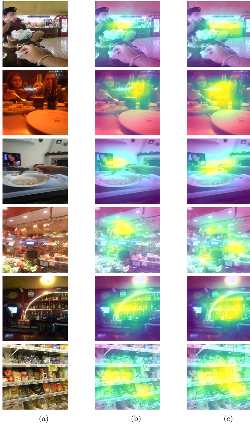
Figure 6.3: (a) Input images, (b) heat maps generated by Grad-CAM for the baseline FT-ResNet50, and (c) heat maps generated by Grad-CAM for the model trained with the proposed training scheme (0-occlusion).
