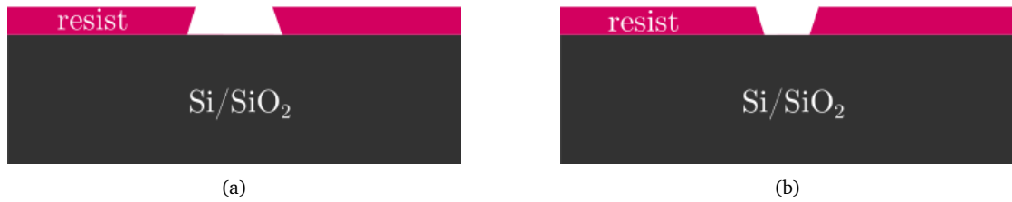
Figure 3.3.: Resist profile illustration of (a) negative and (b) positive resist processing modes after development.
