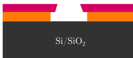
Figure 3.5.: Illustration of the profile of a double layer resist after development. Both, pink and orange, represent the two resists on the resist stack.
