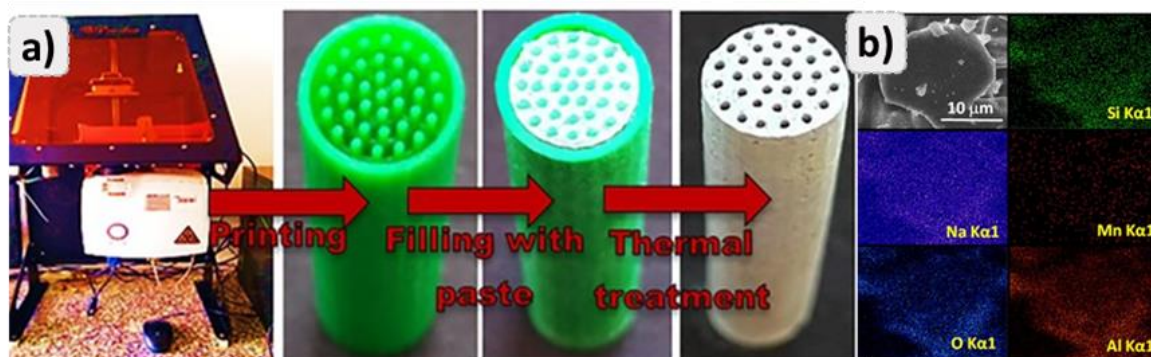
Figure 2.9. Ceramic monolithic catalyst obtained by means of DLP printed templates: a) scheme of production; b) EDS images showing the homogeneous elemental distribution within the monolith channel. Adapted from [107].
