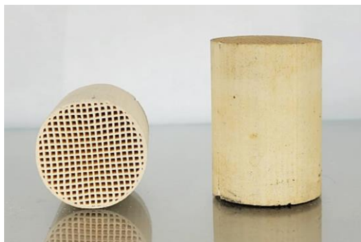
Figure 4.1. Commercial honeycomb cordierite monoliths used for evaluation of CO 2 methanation.
