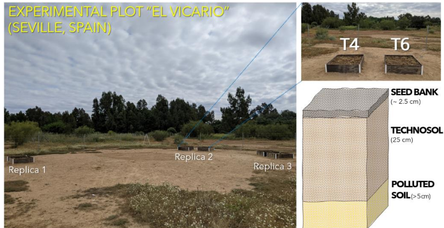
Figure 2.7. View of the experimental plot "El Vicario" in the GGC and the scheme of the combined remediation system for polluted soils.
