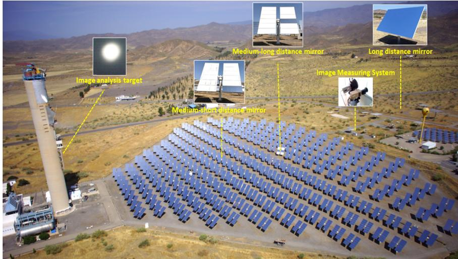
Figure 1: Image acquisition setup at the Plataforma Solar de Almería. From left to right: Image analysis target (where the real projected shapes are measured), Medium-short and Medium-long distance mirror (where the F62 and F42 facets are mounted, respectively), Image measuring system (image acquisition equipment), and Long distance mirror (where the LDM facet is mounted).
