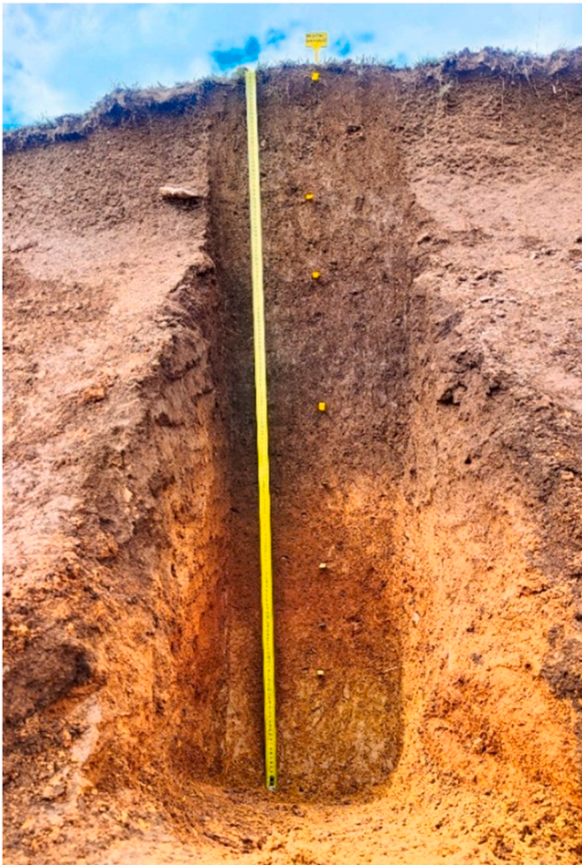
Fig. 2. General aspect of the soil profile derived from the sampling, where the IX (9) identified levels can be distinguished. Source: authors.
