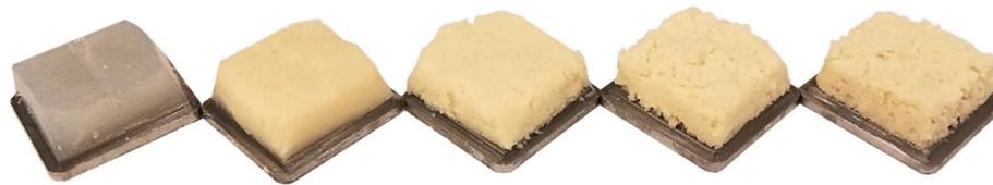
Fig. 1. The visual representation captures the assortment of model foulants subjected to experimentation, arranged from left to right as follows: P0 (100% starch gel), P30, P60, P80, and P100 (100% whey protein gel). These samples are placed on a flat metal surface with dimensions measuring  $2.5 \times 2.5$  cm.
