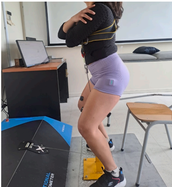
Fig. 1. Measurement of force, power, and sEMG during dynamometric evaluation of the iSTS in a representative female participant.
