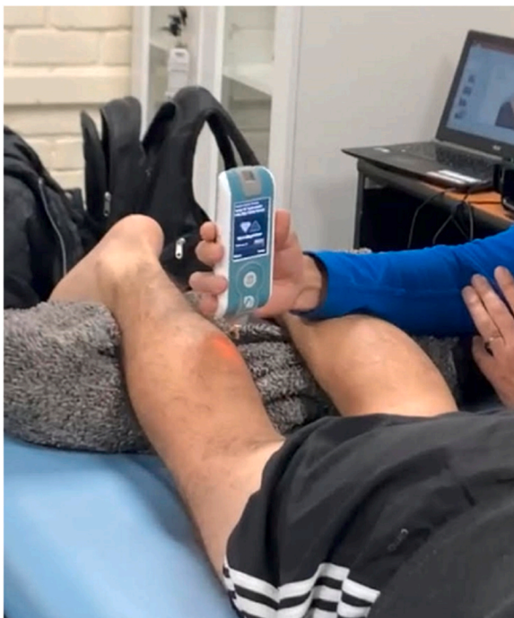
Fig. 2. Measurement of muscle oscillation frequency of the gastrocnemius medialis using a myotonometer in a representative male participant.
