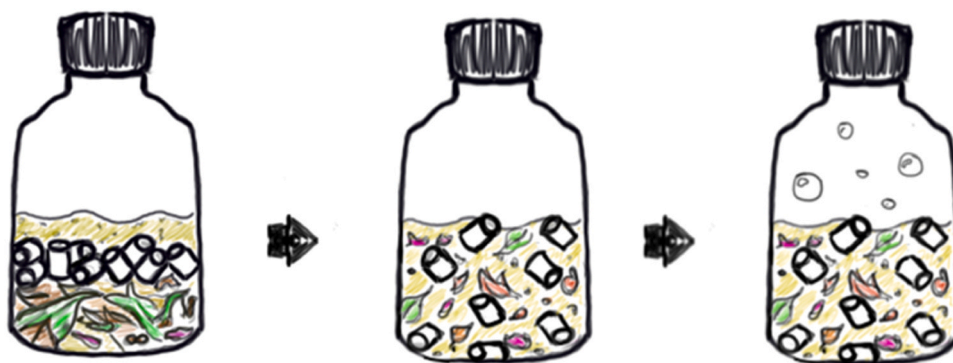
Fig. 1. Bottles drawing during experimental assays: a) preparation (substrate, BA and inoculum), b) after manual mixing and c) start-up after air purging.
