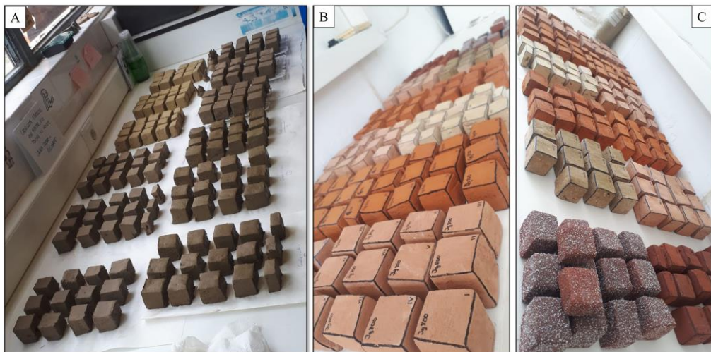
Figure IB-1. Photograph of the bricks studied in this work. A) Unfired bricks made from raw materials from Jun and Guadix with and without household glass; B-C) general view of fired bricks with and without household glass.
