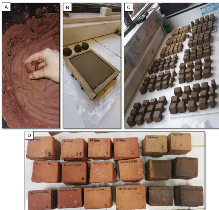
Figure II-S1. Brick making process. A) Raw materials are kneaded with water; B) the kneaded clayey mass is placed in the wooden mould; C) cut samples are left to dry in the laboratory; D) fired bricks: control group (bricks with no added carbon fibre) in the top row, bricks with 5 wt.% carbon fibre in the middle row, and bricks with 10 wt.% carbon fibre in the bottom row.
