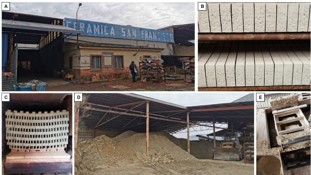
Figure 8. A) Ceramica Castillo Siles factory; B) Drying of extruded bricks; C) Stack of bricks ready for firing in the oven; D) Clayey material piled up outside the factory; E) Moulds used for the production of handmade bricks.
