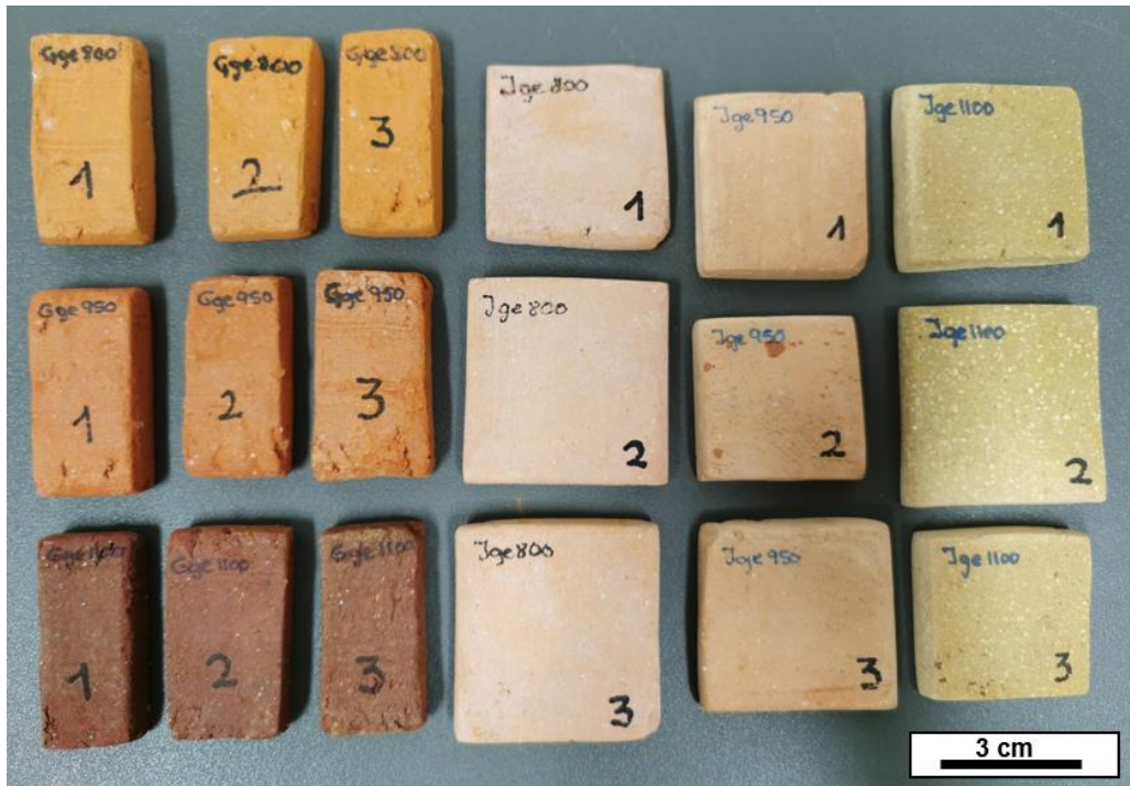
Figure 15. Extruded bricks supplied by the Castillo de Siles brick factory. The bricks on the left, with rectangular shapes and brighter colours, were made with clay from Guadix and household glass powder. The bricks on the right, with square shapes and less luminous colours, were made with clay from Jun and household glass powder.
