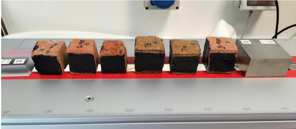
Figure 18. Thermal behaviour of the bricks with tea residue added analysed in the Department of Geosciences at the University of Padua.
