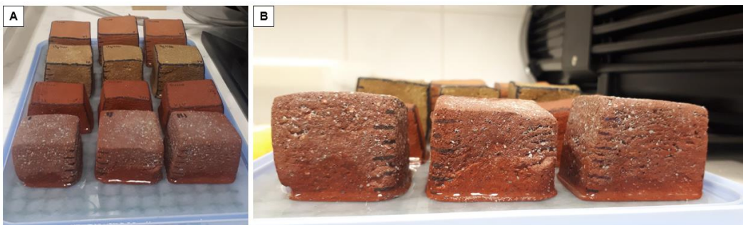
Figure 19. A) Image of the capillarity test carried out on the handmade bricks of Chapter I (bricks from Jun and Guadix with and without added household glass powder); B) capillarity rise in the handmade bricks made with raw material from Guadix with household glass added.
