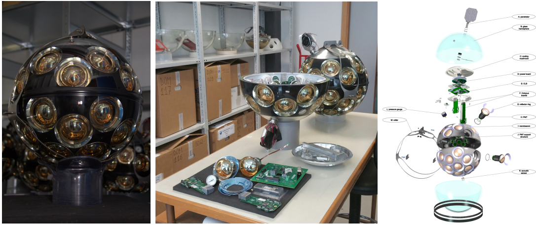
Figure 4.6: Picture of a KM3NeT Digital Optical Module mounted (left) and dismounted (centre), and drawing of a DOM components (right). From KM3NeT homepage [124].
