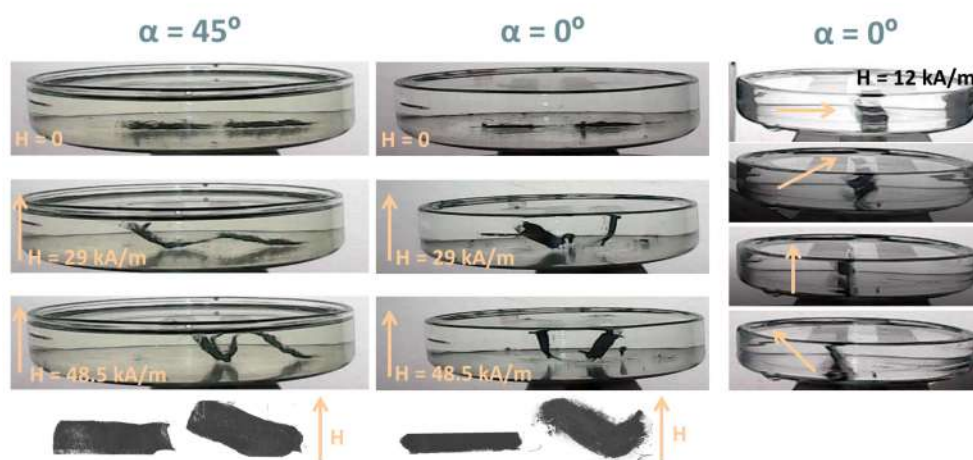
Figura 9.14: Photographs of the worm-shaped actuator with the magnetic parts aligned at 0^\circ and 45^\circ under applied magnetic fields of different intensities or directions. Corresponding microCT images are included for each condition.
