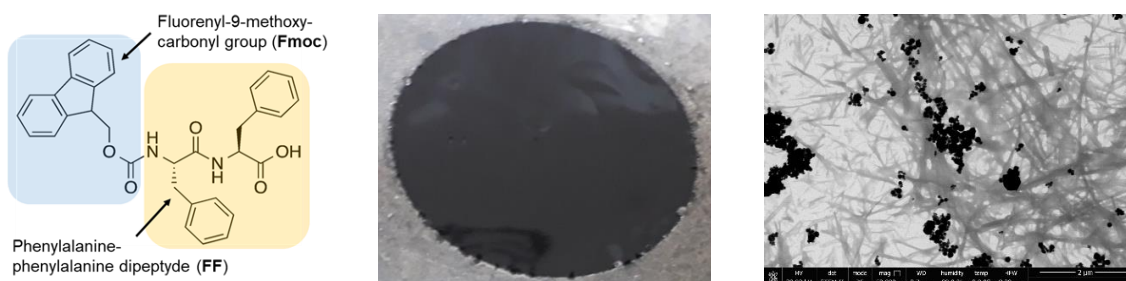
Fig. 1. Formula of Fmoc-FF molecule (left), resulting magnetic hydrogel (center), micrograph of the hydrogel structure by ESEM microscopy; the scale bar is 2 μm (right)
