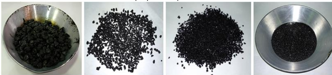
Figure 4.3 2 Disaggregation of asphalt mixture into groups to define the bitumen content employed in asphalt mortars.
