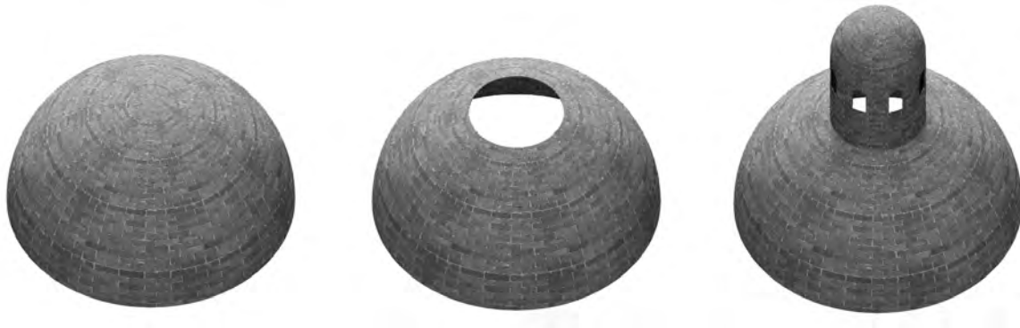
Figure 49 Three structural situations have been considered: full hemisphere, hemisphere with oculus and hemisphere with inside brick coating of lantern.
