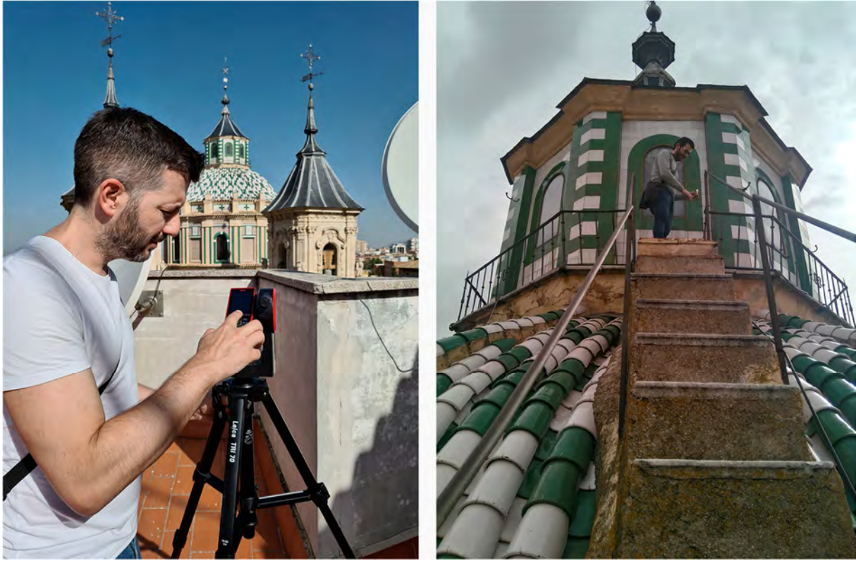
Figure 79 On-site check-up and measurement of the different elements in the dome.
